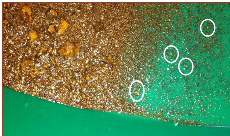
Figure 8. Crushed Iron pisolith sample containing gold grading up to 282 g/t in iron pisolites. (Source: TRP)
